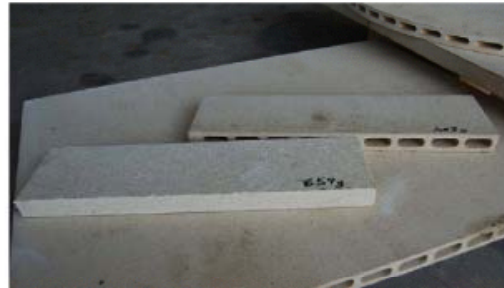
ABOVE, BOTH SHELVES ARE 3" X 10", THE SOLID SHELF IS 3/4" THICK WHILE THE HOLLOW CORELITE SHELF IS 7/8", YET THE CORELITE SHELF IS 24% LIGHTER
